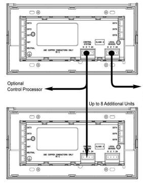
Control system as master with slave wiring
